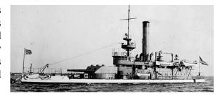
Displacing 3,180 tons, the ARKANSAS' main armament was two 12-inch guns mounted in a single turret. One innovation she enjoyed was the first installation of an electric turning gear for her sole gun turret. Her career was largely limited to coastal protection and as a summer season cruise ship for US Naval Academy midshipmen. Renamed OZARK in 1909, she served as a submarine tender during World War I. OZARK (ex-ARKANSAS) was decommissioned in 1919 and scrapped three years later.
