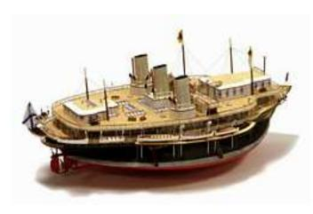
Popov's modified design included a more conventional bow and stern. The result was an odd and somewhat oblong hull shape that was 235 feet in length, with a beam of 153 feet. A large and lavishly furnished superstructure was provided.
